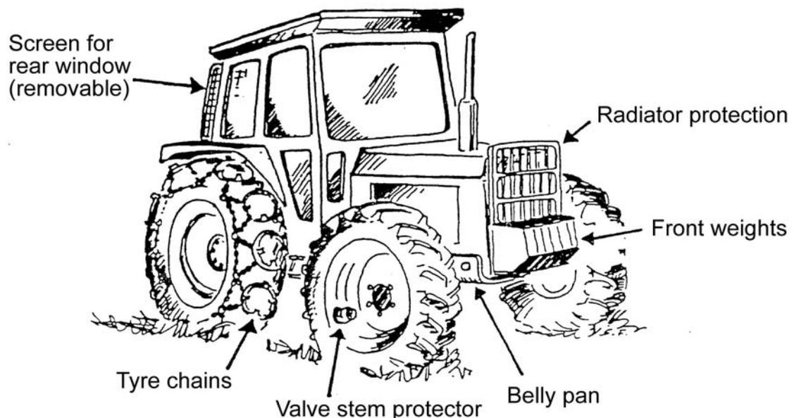
(with a front to rear ratio of 45:55) improves stability and pulling power.
