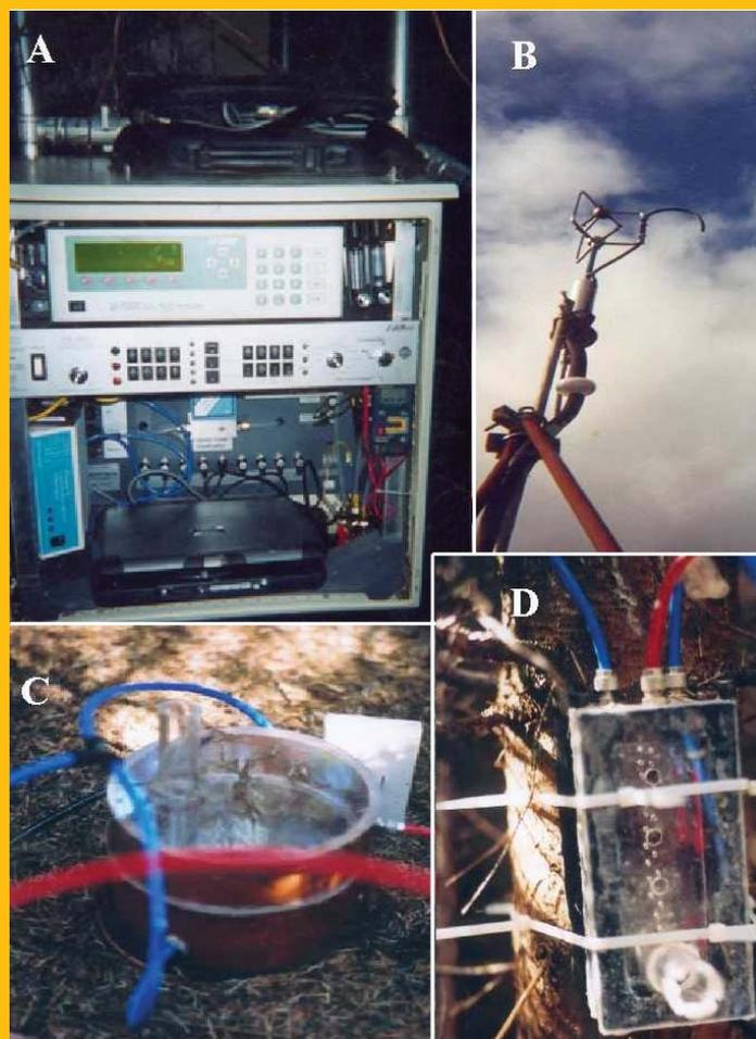
*The eddy covariance system (A, B), soil (C) and bole (D) respiration chambers used for the collection of continuous flux and respiration data.*
