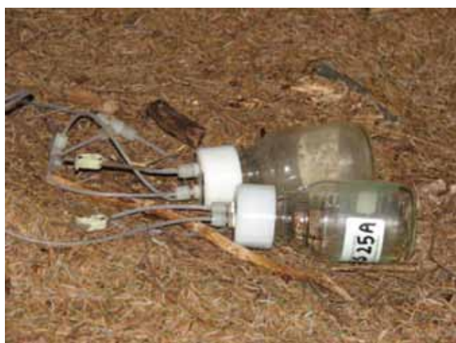
Deep soil water samplers.
