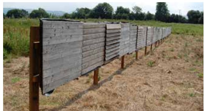
Figure 4: Panel exposure test site near Clonmel, County Tipperary. Also showing the different profiles used to construct the panels.
