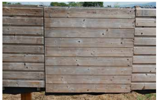
Figure 5: A heat treated Sitka spruce panel after six years of exposure.
