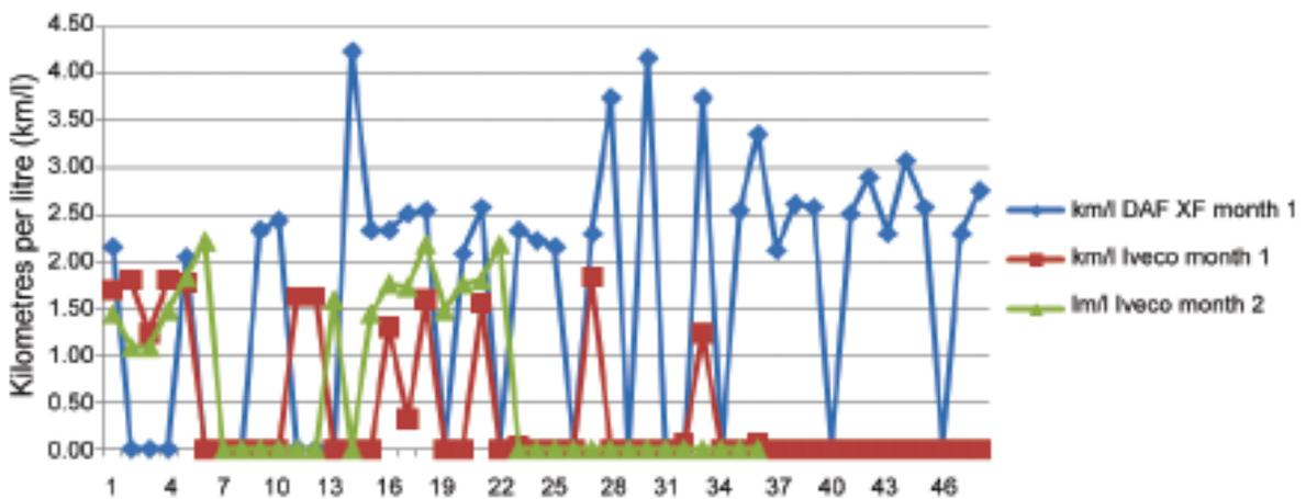
Figure 3: Km/l of Daf XF (general) vs Iveco Stralis (timber).
