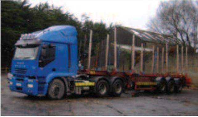
Figure 1: Iveco Stralis 530 articulated configuration.
