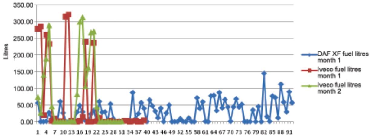
Figure 4: Fuel litres used by Daf XF vs Iveco Stralis.
