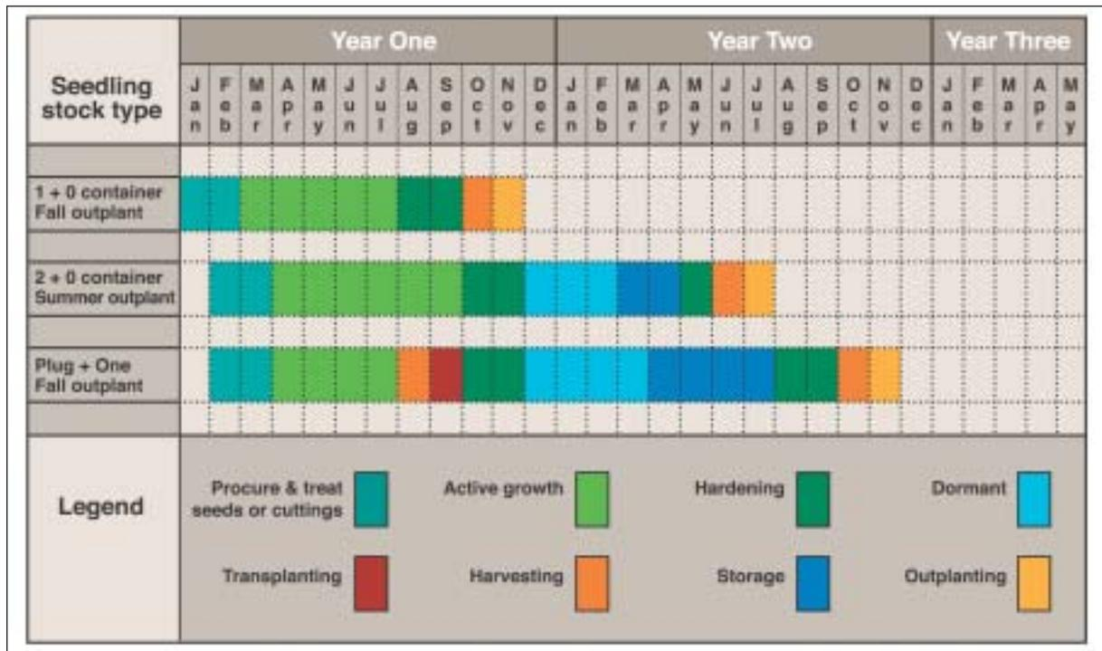
Figure 5: Summer and autumn outplanting are now possible for high elevation or high latitude sites, but the container stock is produced with special nursery production schedules that incorporate special conditioning.
