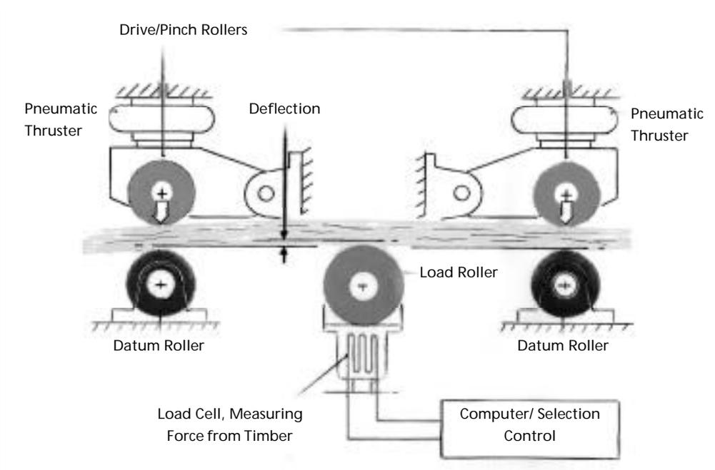
Figure 1: Schematic plan view of three point bending test in the Cook-Bolinder machine.
