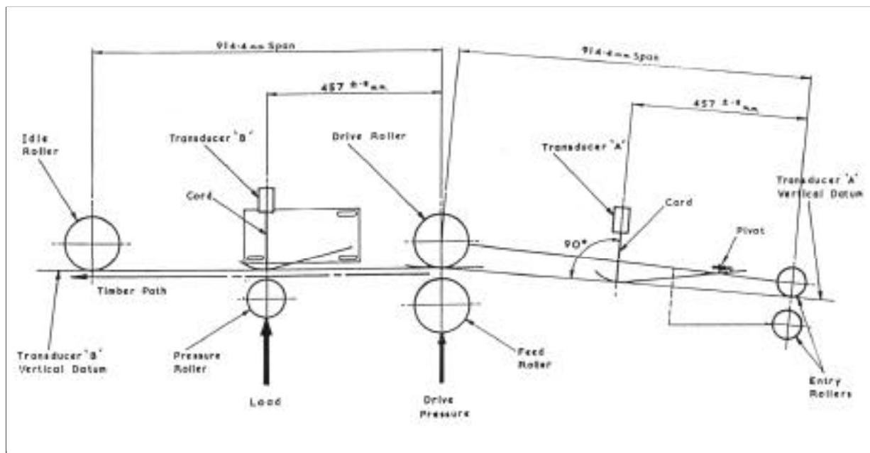
Figure 2: Schematic plan view of three point bending test in the MPC machines (Computermatic and Micromatic)
