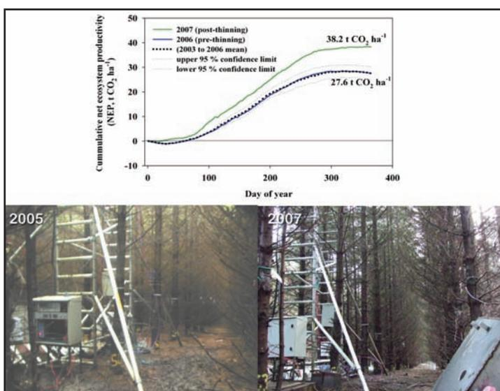
Figure 2: Changes in NEP and canopy characteristics before (2005/6) and after thinning (2007). Positive NEP values (excluding C losses in harvested wood) represent an uptake of CO<sub>2</sub>. Note the reduction in green leaf area after thinning.
