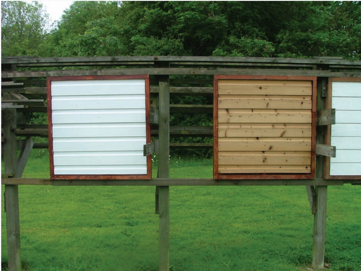
Figure 3: Panels undergoing exposure trials at the Building Research Establishment.
