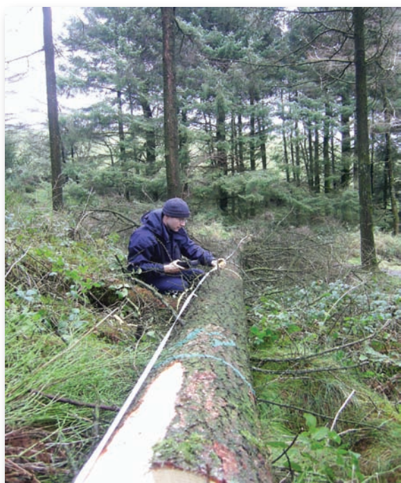
Sectional measurement of a felled volume sample in a STANDMODEL Japanese larch plot, near Virginia, Co Cavan.
