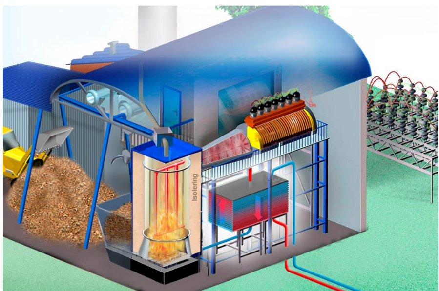
Figure 8: A simplified view of a combined heat and power plant on wood chip (By kind permission of Fjernvarmeskolen.dk).
