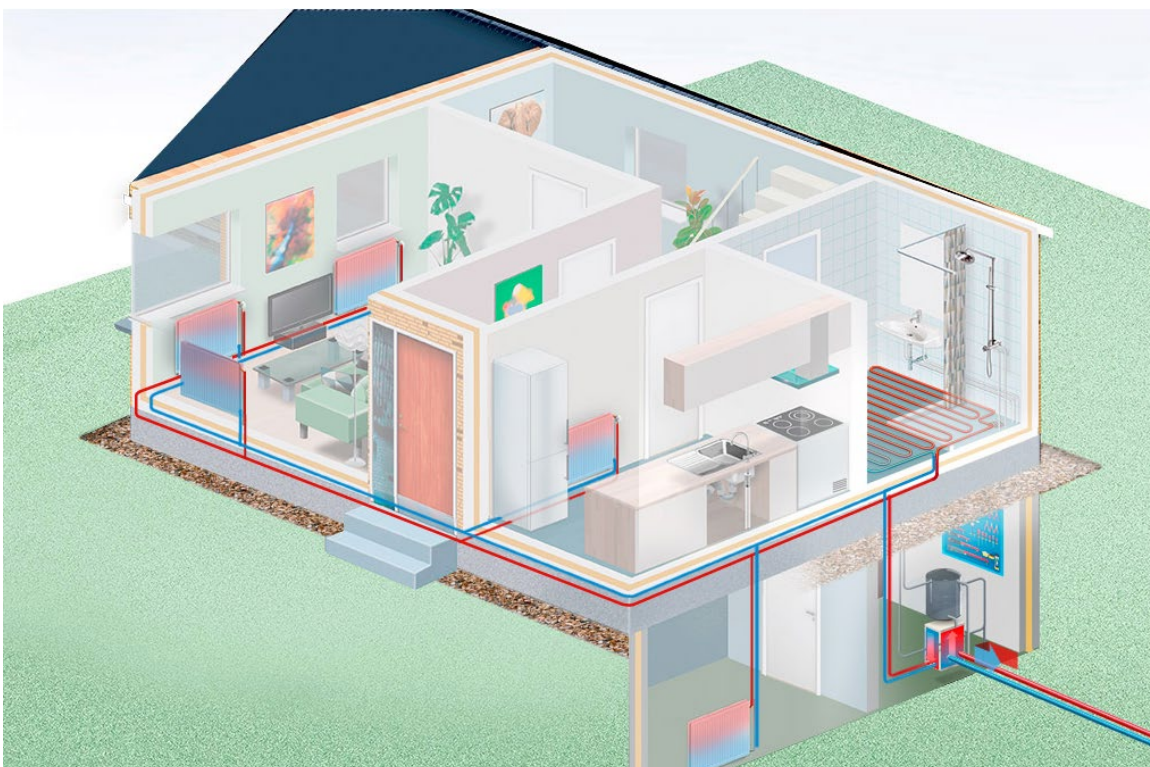
Figure 4: The DH water does not circulate in the house (By kind permission of Fjernvarmeskolen.dk).
